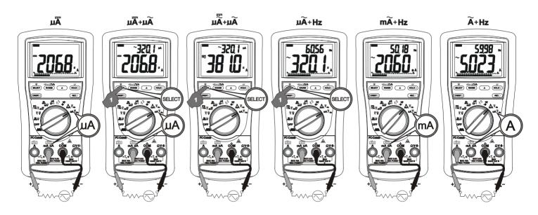
\*Note: When measuring a 3-phase system, special attention should be taken to the phase-to-phase voltage which is significantly higher than the phase-to-earth voltage. To avoid exceeding the voltage rating of the protection fuse(s) accidentally, always consider the phase-to-phase voltage as the working voltage for the protection fuse(s).
