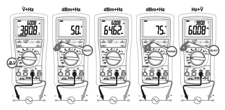
Note: Hz Input sensitivity varies automatically with voltage (current function alike) range selected. 1V range has the highest and the 1000V range has the lowest. Auto-ranging
