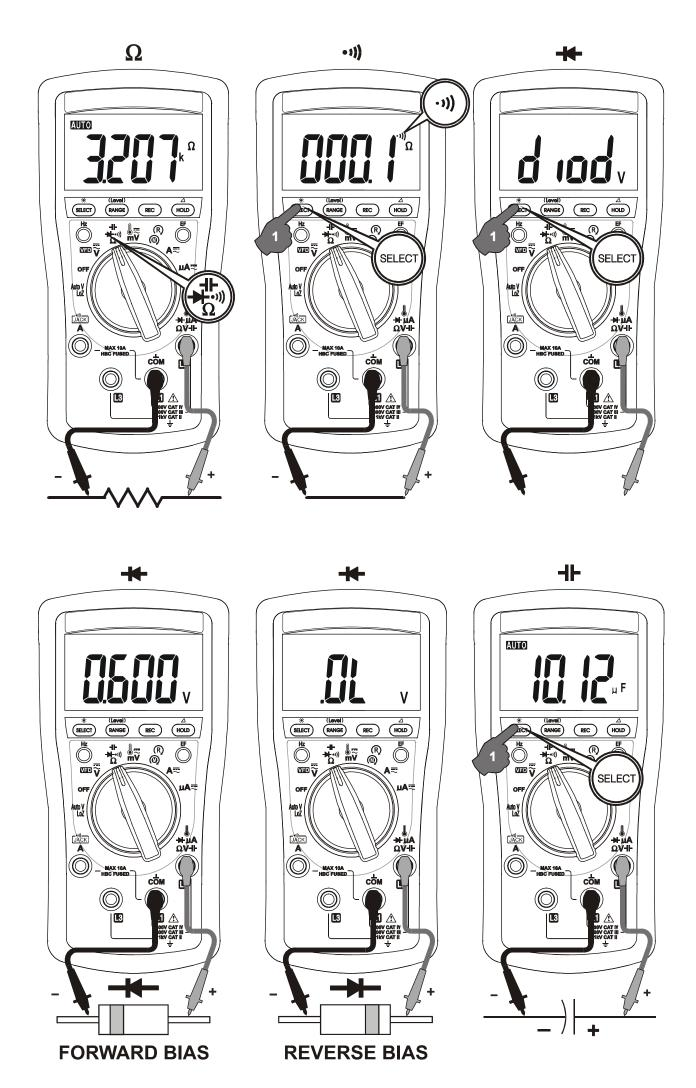
•)) BeepLit<sup>TM</sup> Continuity function is having improved convenience for checking wiring connections and operation of switches. A continuous beep tone together with flashing display backlight indicate a complete wire. Such audible and visible indications improve continuity readabilities in noisy working environments.
